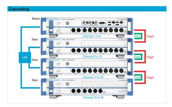
If more than eight channels have to be measured in parallel, several R&S<sup>®</sup>UPP audio analyzers can be cascaded. The master, an R&S<sup>®</sup>UPP800, controls the other audio analyzers, so the entire cascade acts as a single measuring instrument.
