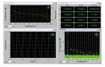
With graphical representations, results can be read off using vertical and horizontal cursors; markers and limit traces make evaluation easier. Multiple traces can be superimposed in user-defined colors.
