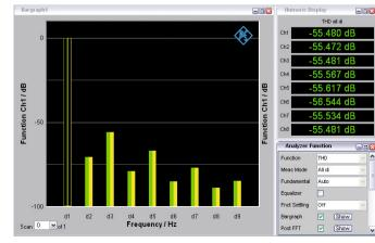
The THD measurement can be used to analyze all, individual or any combination of harmonics.
