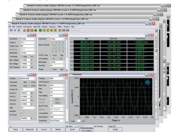
Everything at a glance: Multiple measurement diagrams can be arranged in any desired configuration on the screen; analyses in the frequency and the time domain can be displayed simultaneously.
