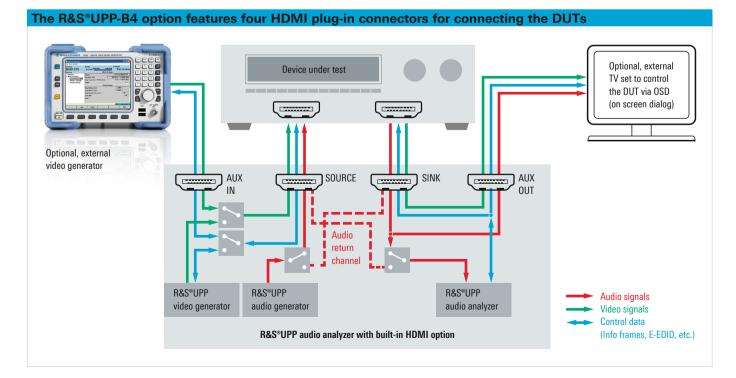
The R&S<sup>®</sup>UPP-B4 option features four HDMI plug-in connectors and two RJ-45 female connectors for the HEC signals.
